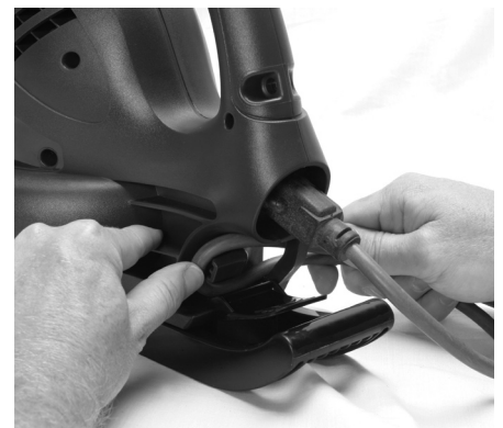
Figure 4-3: Pull extension cord loop tight around molded cord hitch
